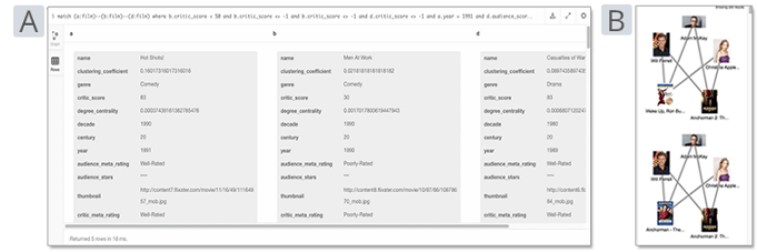
Fig. 2. (A) Neo4j, a commercial system, displays subgraph matches in a long table. One match with three nodes is shown here, each gray box describes one nodes’ features. (B) VISAGE [33] displays subgraph matches in a list, without revealing connections among results. Even for modest sized queries, these conventional approaches require significant scrolling, and cannot easily reveal broader patterns and relationships among matches.
